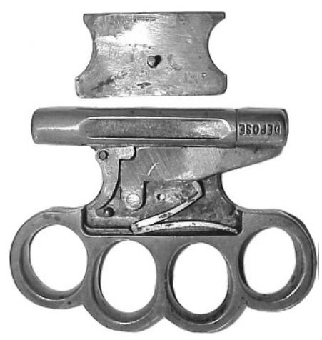
ED. A good view of the action in a "Depose" knuckleduster. On the right note the tiny wire spring that pushes the trigger forward.
